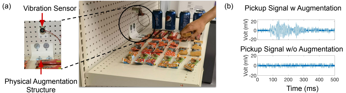
Figure 1: (a) A prototype of our single-point vibration sensing system with the physical augmentation structure. (b) Example signals of the pickup event with and without the physical augmentation.
